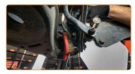
Unscrew the caliper bracket fastening. Use XZN #14.
