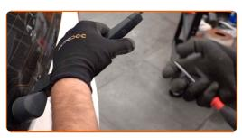
Press the clip. Use a flat screwdriver. Remove the blade from the wiper arm.
