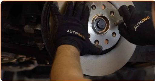
**35** Tighten the brake disc fastening. Use Torx T30. Use a torque wrench. Tighten it to 4 Nm torque.
