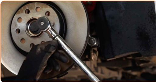
**36** Install the brake caliper together with its bracket.
