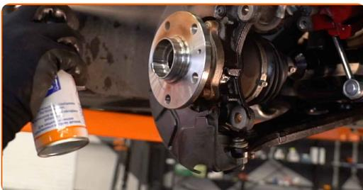
**33** Install and tighten the drive shaft bolt. Use drive 12-point socket #24.
