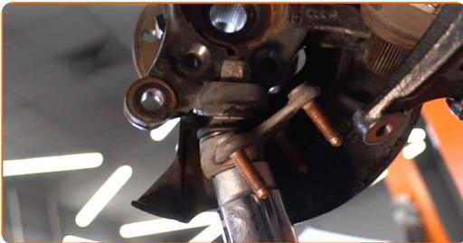
31 Tighten the ball joint fastening nut. Use a drive socket #15. Use a torque wrench. Tighten it to 60 Nm torque.
