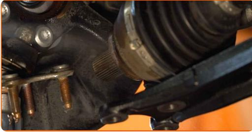
29 Mount the drive shaft into the wheel hub.
