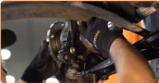
30 Attach the ball joint to the control arm.
