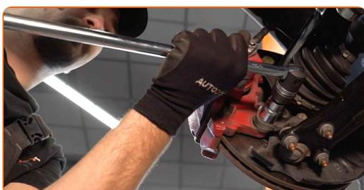
14 Remove the brake caliper together with its bracket.
