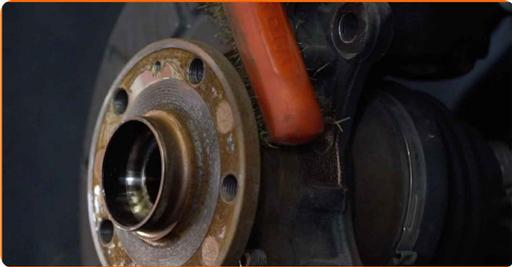
19 Remove the drive shaft from the wheel hub.
