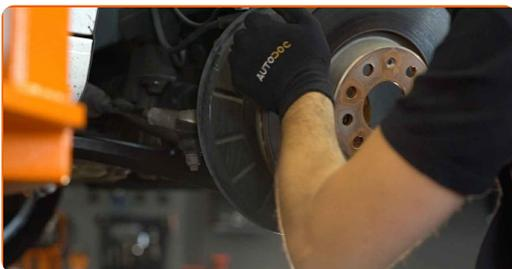
17 Unscrew the wheel hub axle nut. Use drive 12-point socket #24.
