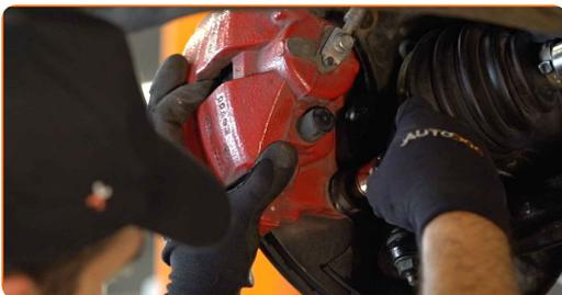
**37** Tighten the brake caliper bracket. Use a drive socket #21. Use a torque wrench. Tighten it to 190 Nm torque.
