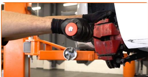
13 Unscrew the caliper bracket fastening. Use a drive socket #21. Use a ratchet wrench. Use a tap wrench.
