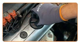
Tighten the oil filler cap.
