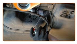
Take the fluid container away from under the fuel filter.
