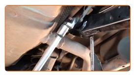
Remove the support from under the arm.
