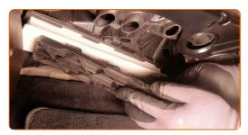
8 Install the bottom cover of the glove box.
