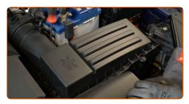
Slightly raise the cover of the air filter housing.
