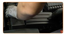
Screw in the fastening screws of the air filter cover. Use Torx T27. Use a ratchet wrench.
