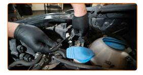
Detach the bulb holder by turning it by ~30°. Remove the holder from the headlight mounting seat.
