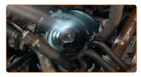
Unscrew the filter housing cap together with the old filter element. Use a drive socket #30. Use a ratchet wrench.
