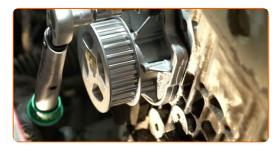
Tighten the water pump fasteners. Use HEX No.H6. Use a torque wrench. Tighten it to 20 Nm torque.
