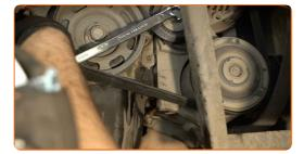
Pull aside the V-ribbed belt tensioner pulley. Use a combination spanner #16.
