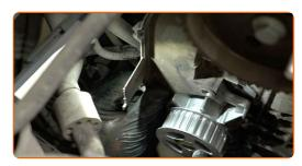
Screw in the water pump fasteners. Use HEX No.H6. Use a ratchet wrench.
