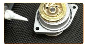
Install the water pump gasket.
