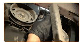
Screw in the fastener of the serpentine belt tensioner pulley. Use a combination spanner #16.
