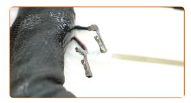
6 Attach the mirror heating connectors.
