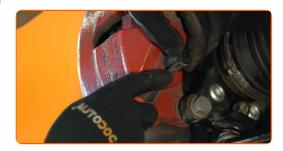
Unscrew the brake caliper fastening. Use HEX No.H7. Use a ratchet wrench.
