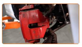
19 Install the brake caliper retaining spring.
