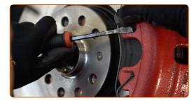
11 Remove the brake caliper.
