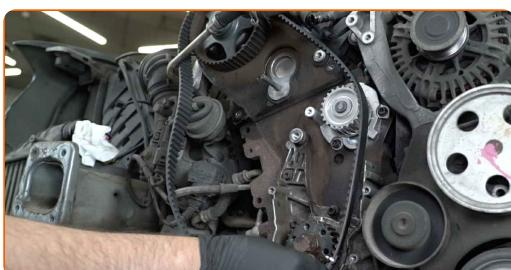
**Replacement: water pump & timing belt kit – VW Golf V Hatchback (1K1). Tip:**
