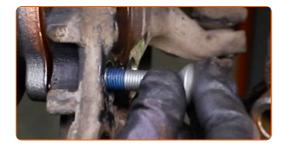
Tighten the wheel hub bolts. Use XZN #12. Use a torque wrench. Tighten it to 70 Nm torque.
