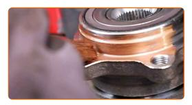
Install the new wheel hub together with the bearing.
