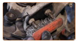
Unscrew the fasteners connecting the ball joint to the control arm. Use a drive socket #16. Use a ratchet wrench.
