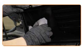
Insert a new filter element into the filter housing.
