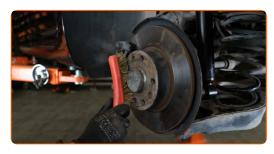
Treat the contacting surface. Use copper grease. 25.2
