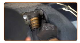
Tighten the shock absorber mount fasteners. Important! Be sure to use new fasteners. Use a drive socket #16. Use a torque wrench. Tighten it to 50 Nm torque.+45°
