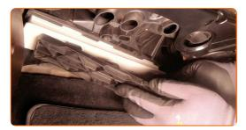
Install the bottom cover of the glove box.
