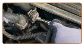
6 Unscrew the brake fluid reservoir cap.
