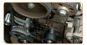
Replacement: water pump + timing belt kit – VW GOLF PLUS (5M1, 521). Tip:
