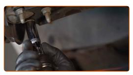
Unscrew the rear fastener connecting the control arm to the subframe. Use a drive socket #15. Use a tap wrench.
