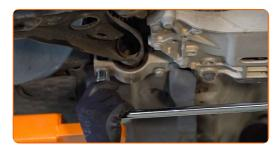
Unscrew the front arm fastener. Use a drive socket #15. Use a drive socket #18. Use a tap wrench.
