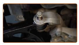
Attach the ball joint to the control arm.
