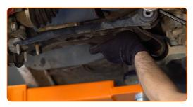
Treat the fasteners of the ball joint. Use copper grease.
