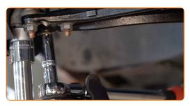
Remove the support from under the arm.
