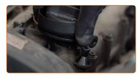
Attach the crankcase ventilation hose to the oil filler neck.
