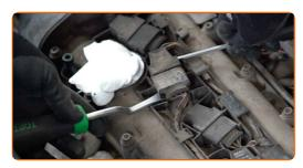
Undo the plastic locking tabs of the ignition coil connector. Use a flat screwdriver.
