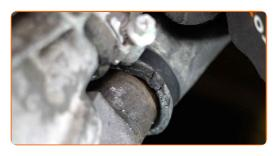
Drain the coolant from the engine.
