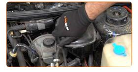
Remove the fender protection cover.
