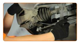
Loosen the fastener of the driveshaft. Use a drive socket #30. Use a ratchet wrench.
