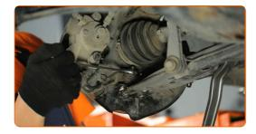
Install the rod fastening to the stabilizer and tighten it. Use a drive socket #16. Use a torque wrench. Tighten it to 15 Nm torque.+90°
