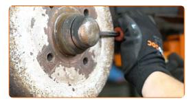
Remove the cotter pin securing the hub nut. Use a crowbar.
