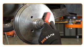
Treat the surface where the wheel rim contacts the brake drum. Use copper grease.
