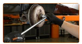
Remove the brake drum assembled with the wheel hub bearing. Use a flat screwdriver.
