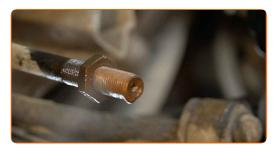
Screw on a new tie rod end. Use a vernier caliper.
