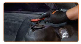
Loosen the upper fastener of the shock strut mount. Use a combination spanner #17. Use a shock absorber socket DDNº6. Use a ratchet wrench.
