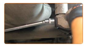
11 Remove the fastening bolt.
