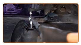
Treat the upper fastener of the suspension strut mount. Use copper grease.
