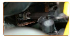
9 Remove the secondary air pump bracket.
