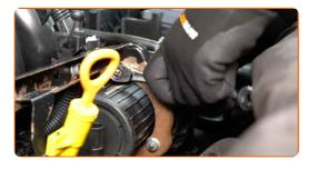
Remove the secondary air pump.
