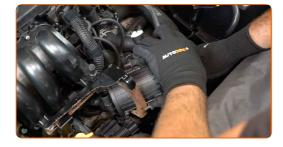
Unscrew the fastener of the secondary air pump bracket. Use HEX No.H6. Use a drive socket #13. Use a ratchet wrench.
