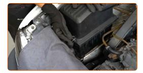
Remove the fender protection cover.
