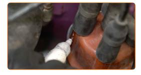
Disconnect the spark plug wires from the distributor cap.
