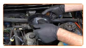
Pour coolant in the coolant reservoir.
