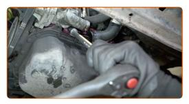
Remove the thermostat housing.
