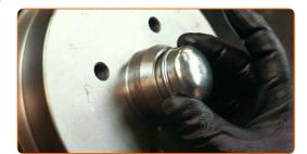
Treat the surface where the wheel rim contacts the brake drum. Use copper grease.
