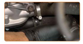
Secure the coolant hose clamp. Use a drive socket #7. Use a ratchet wrench.
