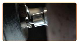
Clean the alternator fasteners. Use a wire brush. Use WD-40 spray.
