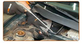
Remove the microfibre cloth from the cabin filter air ducts.
