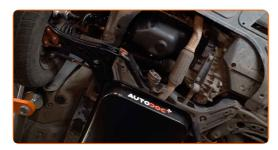
6 Unscrew the drain plug. Use a combination spanner #19.
