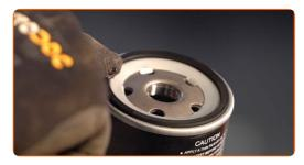
Screw the new filter into its place. Use a drive socket #30. Use a torque wrench. Tighten it to 25 Nm torque.
