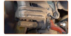
Unscrew the brake caliper fastening. Use a combination spanner #13.
