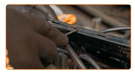
Make marks on the distributor cap to indicate the installation order of the spark plug wires.
