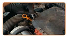
Remove the air filter housing.
