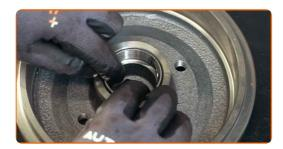
Install the new inner race of the wheel bearing into the brake drum. Use a bush and bearing driver set. Use a hammer.
