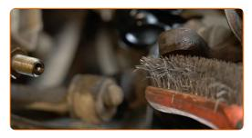
Treat the mounting seats of the tie rod end. Use copper grease. 13
