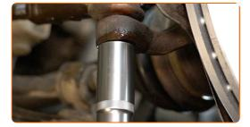
Disconnect the tie rod end from the steering knuckle. Use a ball joint puller.
