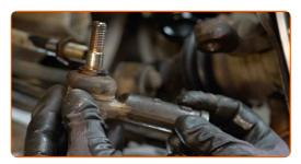
Clean the mounting seats of the tie rod end. Use a wire brush. Use all-purpose cleaning spray. 12
