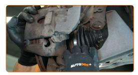
Attach the ball joint to the control arm. Use a pin punch.
