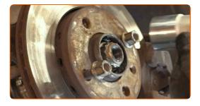
Screw in the nut of the CV axle. Use a drive socket #30. Use a ratchet wrench.
