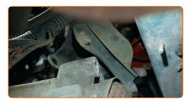
Unscrew the fasteners that connect the gearbox to the engine block. Use a drive socket #18. Use a ratchet wrench.
