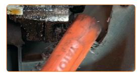
Unscrew the fasteners that connect the bottom gearbox mount to the gearbox. Use a combination spanner #16.
