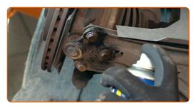
Unscrew the fastener connecting the ball joint to the suspension control arm. Use a drive socket #13. Use a ratchet wrench.
