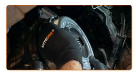
Screw in the pressure plate fasteners. Use 12-point socket No.9. Use a ratchet wrench.
