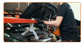
Tighten the fasteners that connect the gearbox to the engine block. Use a drive socket #18. Use a torque wrench. Tighten it to 64 Nm torque.
