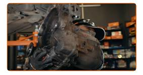
Remove the release bearing. Use a crowbar.
