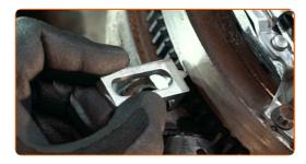
Tighten the pressure plate fasteners. Use 12-point socket No.9. Use a torque wrench. Tighten it to 27 Nm torque.
