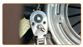
Install the engine flywheel locking tool. Use a clutch tool kit.
