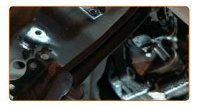
Support the gearbox. Use a hydraulic transmission jack.
