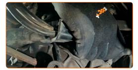
Unscrew the engine starter fasteners. Use a drive socket #13. Use a ratchet wrench.
