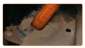
Unscrew the gearbox mount fasteners. Use a drive socket #18. Use a ratchet wrench.
