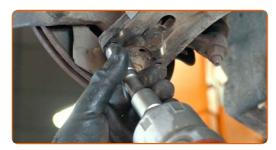
Tighten the fasteners of the CV axle inner joint. Use XZN #8. Use a torque wrench. Tighten it to 42 Nm torque.
