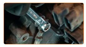
Unscrew the ground wire fastener. Use a combination spanner #13.
