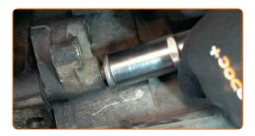
Tighten the fasteners that connect the gearbox to the engine block. Use a drive socket #18. Use a torque wrench. Tighten it to 64 Nm torque.
