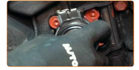
Unscrew the pressure plate fasteners. Use 12-point socket No.9. Use a ratchet wrench.
