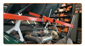
Unscrew the fastener of the cable bracket. Use a combination spanner #16.
