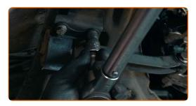
Tighten the fasteners that connect the gearbox mount to the gearbox. Use a combination spanner #16. Use a drive socket #16. Use a torque wrench. Tighten it to 75 Nm torque.
