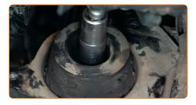
Tighten the fasteners that connect the gearbox mount to the car body. Use a drive socket #13. Use a torque wrench. Tighten it to 38 Nm torque.
