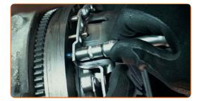
Align the clutch disc. Use a crowbar.
