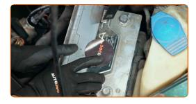
Screw in the battery fastener. Use a drive socket #13. Use a ratchet wrench.
