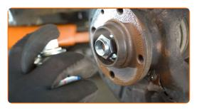
64 Install the brake disc.
