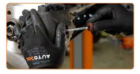
Remove the brake caliper.
