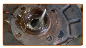
Release the vice and remove the steering knuckle assembled with the wheel hub.
