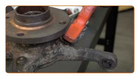
Install the brake disc cover.
