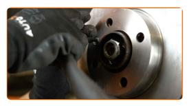
15 Remove the brake disc.
