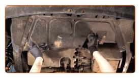
Tighten the fasteners of the oil pan lower cover. Use Torx T20. Use a ratchet wrench.
