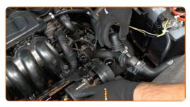
Cover the secondary air pump channels with a microfibre cloth to prevent dust and dirt from getting inside.
