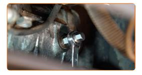
Screw in the new drainage plug and tighten it. Use HEX No.H17. Use a torque wrench. Tighten it to 29 Nm torque.
