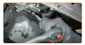
Remove the thermostat housing.
