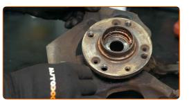
42 Screw in the fasteners of the brake disc cover. Use a drive socket #8. Use a torque wrench. Tighten it to 5 nm torque.
