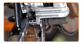
Remove the brake caliper.
