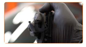
Remove the blade from the wiper arm.
