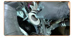
17 Remove the water pump pulley.
