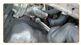
Remove the thermostat housing.
