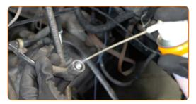
Connect the spark plug wires to the distributor cap.
